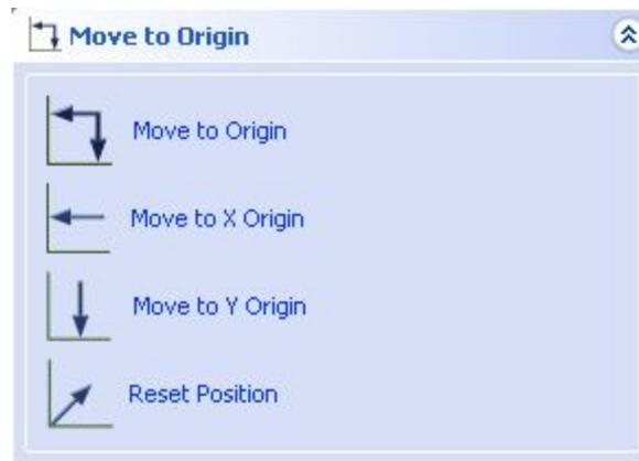
**NOTE:** Moving the part to the origin in FabCreator is different from where on the machine the part will be cut. The origin in FabCreator will end up being the lower-left corner of the “bounding box” for the part. The part itself can still be placed anywhere on the bed of the machine by jogging the cutting head.
