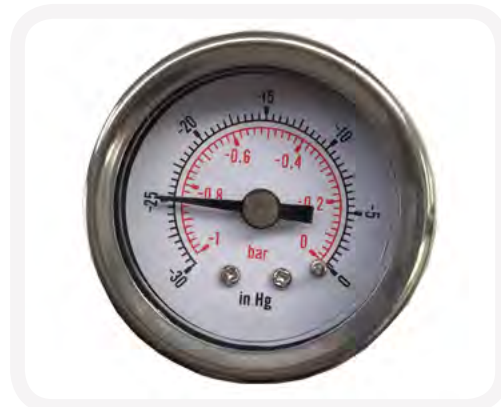
If the vacuum gauge reading of 25" or higher is normal. A lower reading indicated poor vacuum where attention is required.
