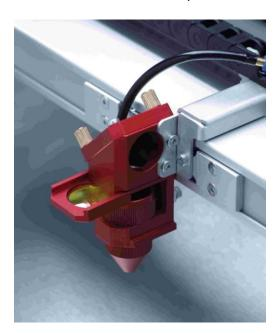
In the Trotec JobControl the lens must be selected under Settings>Options>Engraver or in the symbol bar "Laser Position" to make the autofocus work correctly.
