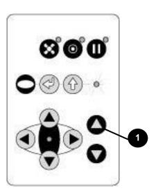
Before the focus tool reaches the work piece, move the working table upwards only very slowly and step by step by briefly tapping the positioning key, until the tool tilts to the side. Now the lens is focused onto the surface of the material.
