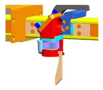
To be able to work with this lens a longer focus tool is needed. Also in JobControl the 2.5" lens must be selected under "Settings > Options > Engraver" or in the symbol bar "Laser Position" to make the autofocus work.
